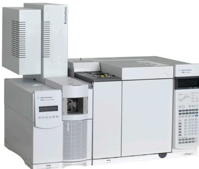
**Triple Quadrupole GC-MS/MS System**
